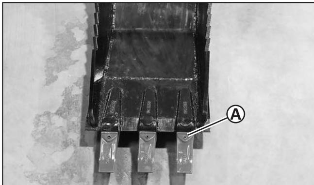
2. Remove the slotted spring pin (A) and the tooth.
