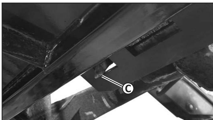
*Picture Note: Wedge on left side of attachment shown. Check the wedges or pins on both sides of the attachment.*
