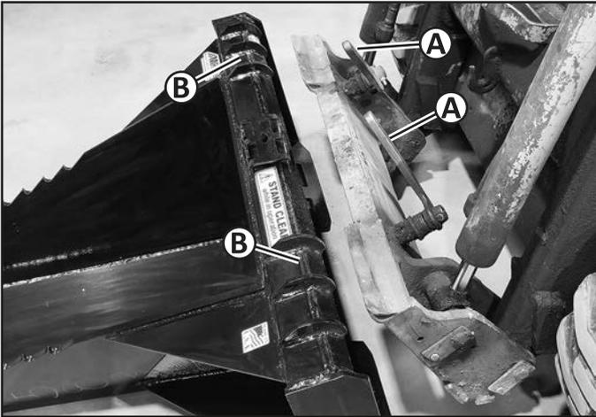
3. Move the loader attaching plate levers (A) to the unlocked (up) position as shown either manually or by using the loader controls.
