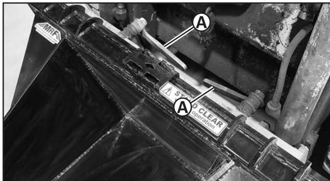
7. Move the loader attaching plate levers (A) to the locked (fully down) position either manually or by using the loader controls.
