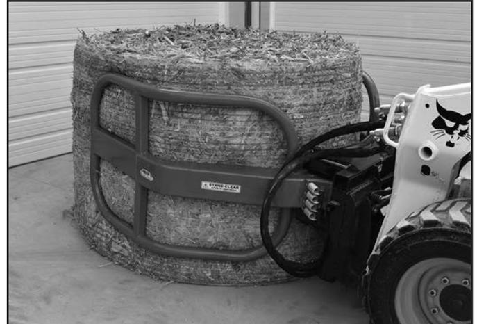
3. Raise the loader lift arms to position the attachment arms around the middle of the bale.
