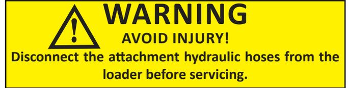
3. Disconnect the attachment hydraulic hoses from the loader.
