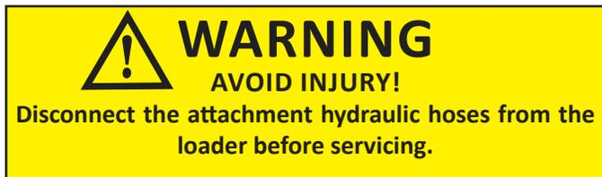
3. Disconnect the attachment hydraulic hoses from the loader.
